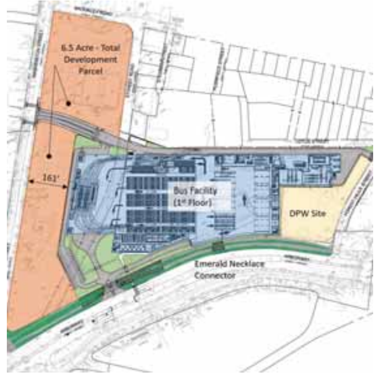
The plan of the proposed Arborway bus garage showing DPW yard and 6.5-acre development parcel.
