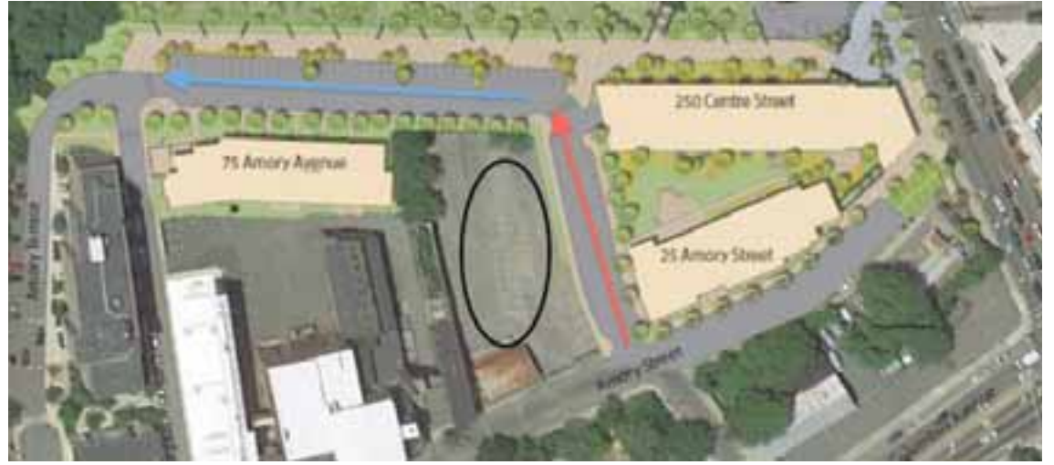
Layout of planned Jackson Square III development. Line in red is the perpendicular road that is debated as a public street. Blue line denotes private way with public use. The oval is 41 Amory St. The white buildings at lower left are BCV properties.
