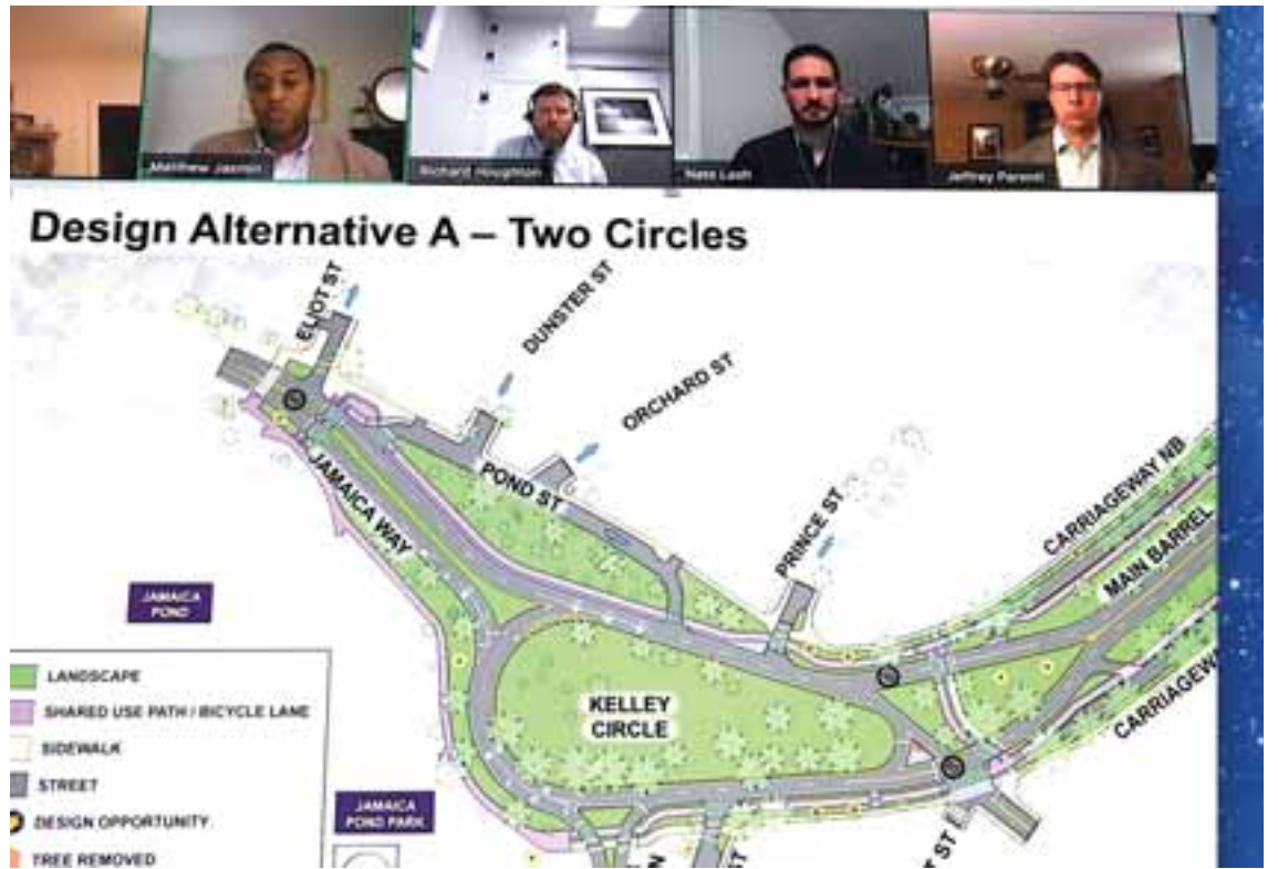
Matt Jasmine (L) project manager and Jeff Parenti, chief engineer (far right), discuss the two circle option, which would maintain both rotaries, but redesign Murray Circle as a much smaller roundabout.
