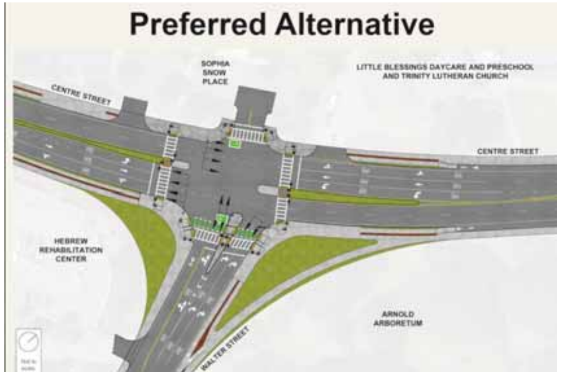
The preferred design will give a dedicated left turning lane for those entering Sophia Snow and a separated bike lane for cyclists coming off of Walter onto Centre towards Jamaica Plain.
